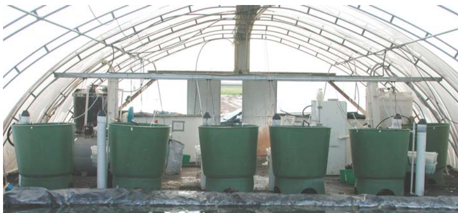
Figure 1. Six tanks with their own recirculating biological filters were used to perform the mullet growth experiments in the sedimentation polytunnel.
